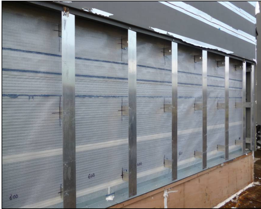
SUPPORT RAILS AT BASE OF SAMPLE
