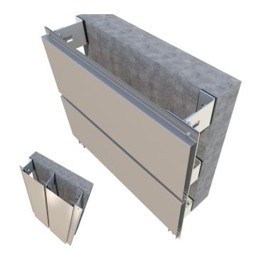
The Matrix IP system can be roll formed or CNC pressed. Panels are manufactured with an external skin of a light gauge material such as CORTEN®, aluminium or zinc and these are generally supplied as 0.8-2mm thick, but this is dictated by the material used.
